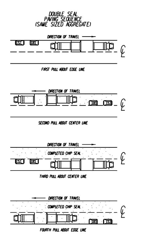
Figure 17. Double Seal Paving Sequence (Same Sized Aggregate).
