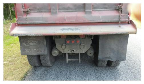
Figure 6. Dump Truck Hitch.
