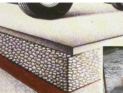
Stores STORMWATER in an aggregate layer to enable infiltration. If water cannot infiltrate, then it can be detained & released.
